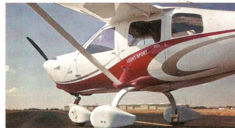
A center control allows entry into the Jabiru (left). The landing gear (below) is made of fiberglass. A separate baggage door (bottom) and roomy baggage area (bottom left) set the Jabiru apart from other LSAs.
