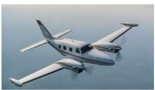
The Mobile ARFF Simulator started life as a Piper PA-31T, PAY1 "Cheyenne I". The PAY1 is a seven-seat cabin class twin engine turboprop. The aircraft was pressurized and routinely flew at altitudes of 18,000 – 30,000 feet. It cruised at approximately 365 knots. The maximum takeoff weight was 9,000 lbs. The PA-31T carried 382 gallons of Jet A (Turbine Engine) fuel.
