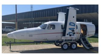
The Mobile ARFF Trainer is an actual Piper PA-31T, PAY1 "Cheyenne I". The PAY1 is a sevenseat cabin class twin engine turboprop. The Mobile ARFF Trainer's empennage has been removed so it can be trailered to off airport locations.
