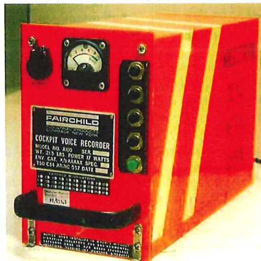
Figure 2. Representative Cockpit Voice Recorder
